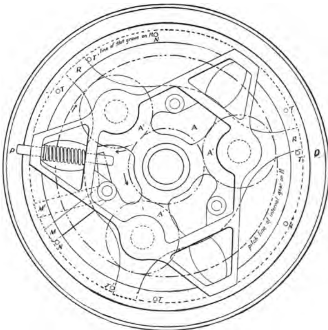
FIG. 270.—Front Elevation of the Duryea Change Speed Gear. The lettering here refers to the same parts as in figure 271, page 380. N marks the position of the lever, M , when pins, P , are inserted in holes, Y , in D . M' marks the position of lever, M , when pins, P , are raised from holes in D . R and R' , arms of the spider, carrying the three idler pinions, A' , and sliding in a groove on H to the pins, T and T' .
